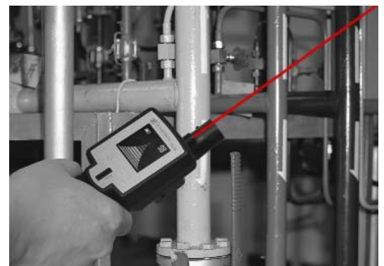
The integrated laser facilitates the detection of leaks
