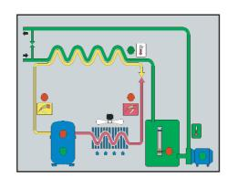
the position of the outlet valve. The Ultracool condenser and evaporator are very oversized in order to achieve the maximum fridge efficiency and reduce power consumption.
